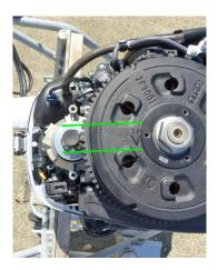
7. Turn the AC generator rotor anticlockwise so that the arrow is lined up with the starter motor as shown.
