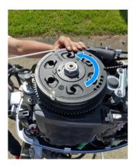
Wind the emergency starter rope clockwise 3 times around the fly wheel along the groove in the ACG rotor.
