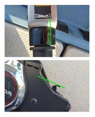
Tiller handle type: Align the "start" mark on the throttle grip with the projected end of the "▲" mark on the tiller handle.
