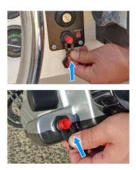
11. Insert the emergency clip into the emergency stop switch. Attach the other end of the emergency stop switch lanyard securely to the operator.
