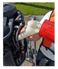
Refill to the upper level mark on the oil level dipstick with the recommended oil. Do not overfill. Too much engine oil may adversely affect the engine.
