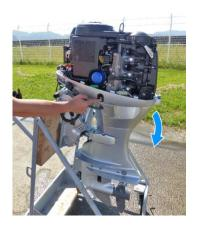
8. Tilt the outboard motor down.
