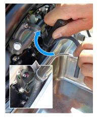
6. After draining, tighten the drain screw.
