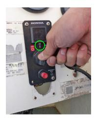
Turn the engine switch key to the ON position.
