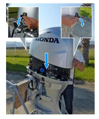
14. Leave the AC generator cover off and install the engine cover. Lock the engine cover fixing levers.
