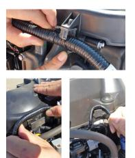
Remove the band clamp, harness and clamp bracket from the ACG cover. Then re-install on the engine side.
