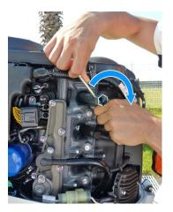
Carefully install the spark plugs by hand to avoid crossthreading. Tighten 1/8—1/4 turn after the spark plug seats. Install the ACG cover.
