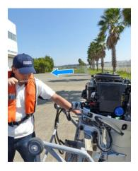
Pull the starter rope lightly until resistance is felt, then pull firmly.
