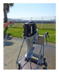
Rinse the outboard motor with fresh water to remove salt water, sand, mud, etc.
