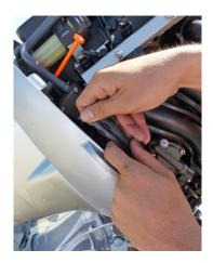
7. Secure the drain tube to the projection of the intake manifold.
